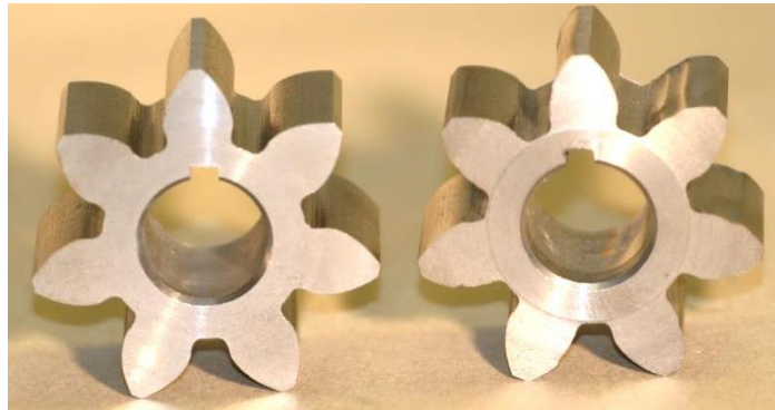
From left to right: A gear with no wear, a worn out gear that needs replacement
