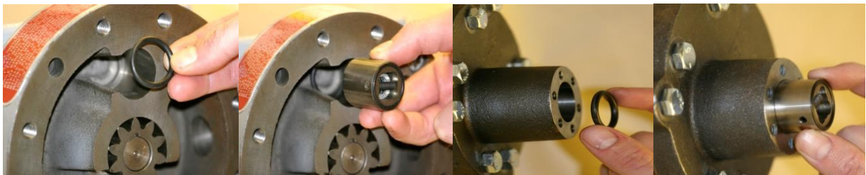
6227-17 o-ring inserted first into E-series main housing
