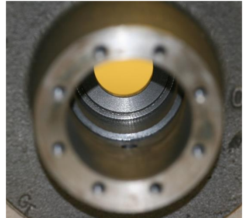
Main housing where shaft seal assembly and bleeder hole is located
