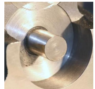
Idler gear shaft in good condition
