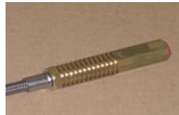
Coupling Failure (Valves are closed by separation and/or back pressure)
