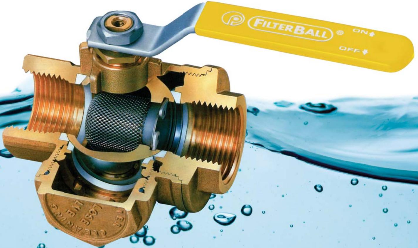
This unique Filter Ball® valve design replaces two standard shut-off valves and a separate strainer. The strainer is readily accessible for cleaning through a screw plug in the valve body after closing the ball valve. The Filter Ball® valve requires less space for installation, lower material and install costs. The Filter Ball® Valve is recommended wherever a shutoff valve and strainer are required.
